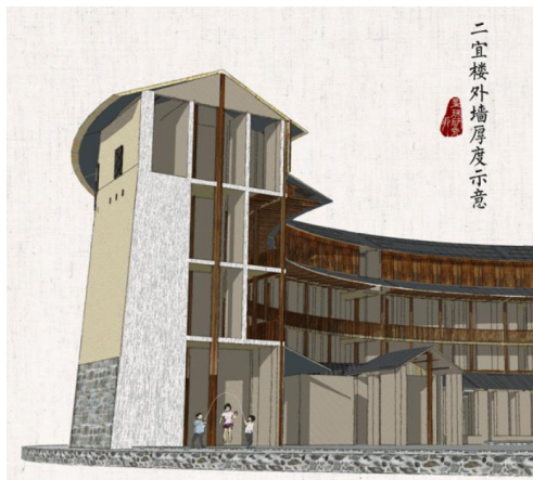
c. Sectional drawing of an earth building (From the network)
