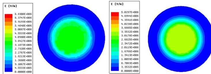
**Figure 10. Comparison of Cloud Images before and after Optimization of Contact Gap Electric Field**
