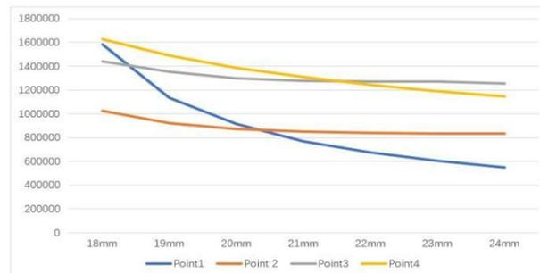
**Figure 8. The Relationship between the Electric Field Strength of the Four Measurement Points and the Size of the Main Shield**
