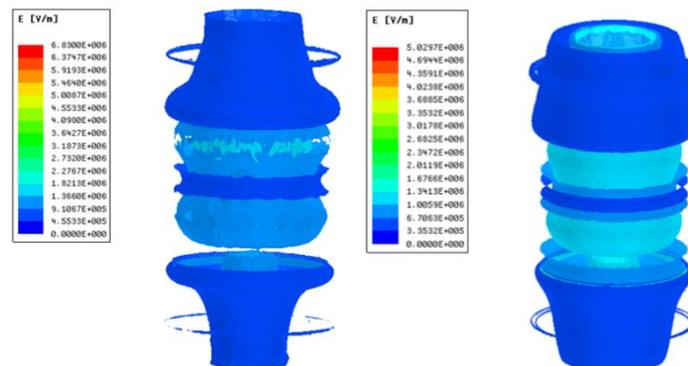
**Figure 9. Comparison of 3D Electric Field Distribution before and after Optimization**
