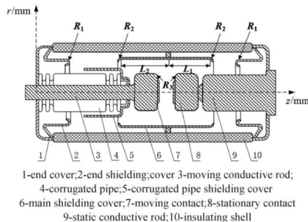
**Figure 1. Physical Model of the Vacuum Interrupter**
