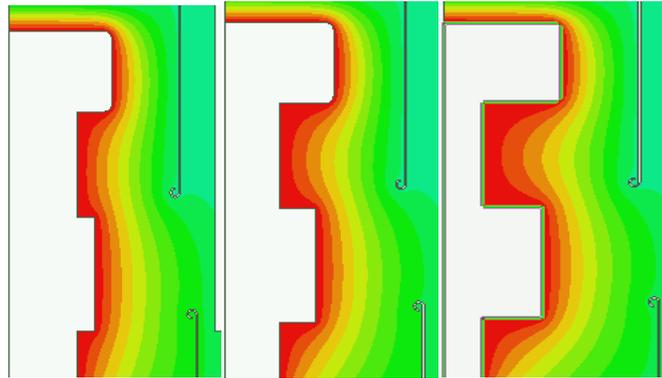
**Figure 4. Influence of Radius of Conductive Rod on Potential Distribution**
