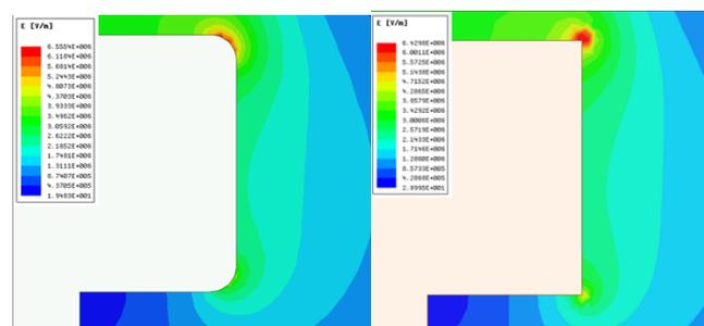
**Figure 3. Electric Field Distribution around Static Contacts**
