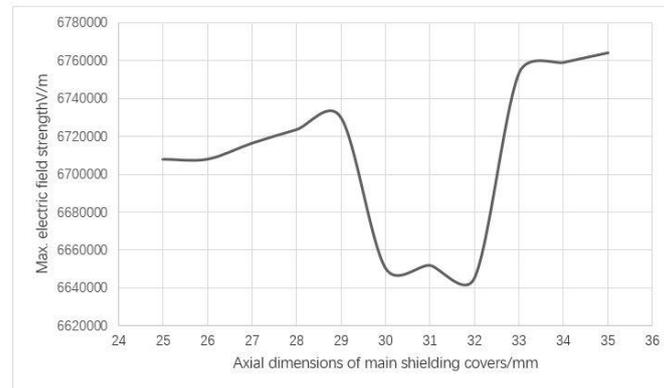
**Figure 6. The Relationship Curve between the Axial Size of the Shield and the Maximum Electric Field Strength**
