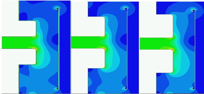
**Figure 5. Effect of Contact Thickness on Electric Field Distribution**
