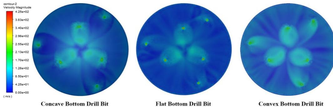
**Figure 6. Bottom Flow Field Velocity Maps for Different Bit Bottoms**
