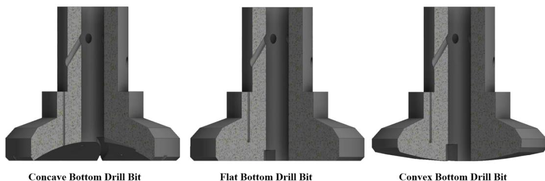
**Figure 2. Three-Quarter Section Views of Bits with Three Different Bottom Structures**
