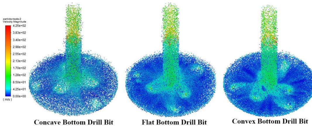
**Figure 9. Particle Velocity Distribution in the Flow Domain**
