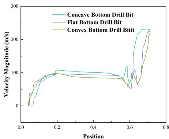
**Figure 5. Axial Air Velocity Distribution in Central Passage for Different Bit Bottoms**
