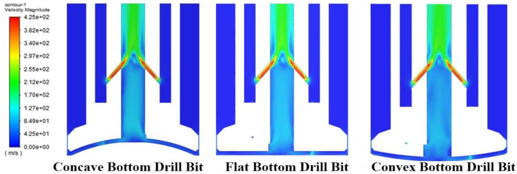
**Figure 4. Internal Cross-Sectional Velocity Cloud Maps under Different Bit Bottom Structures**
