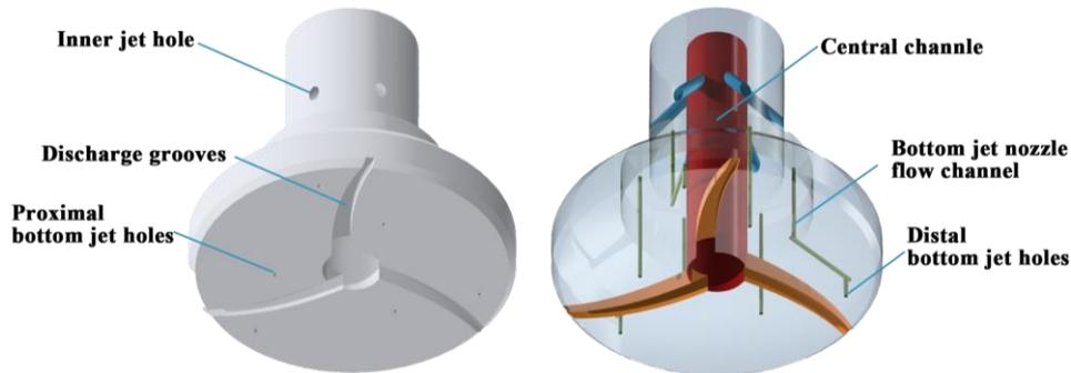
**Figure 1. Perspective View of the Bit's Overall and Internal Structure**
