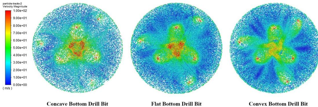
**Figure 8. Particle Velocity at Hole Bottom for Different Bit Bottoms**
