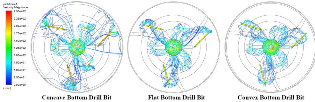
**Figure 7. Streamline Plots of Air Velocity for Different Drill Bit Structures**
