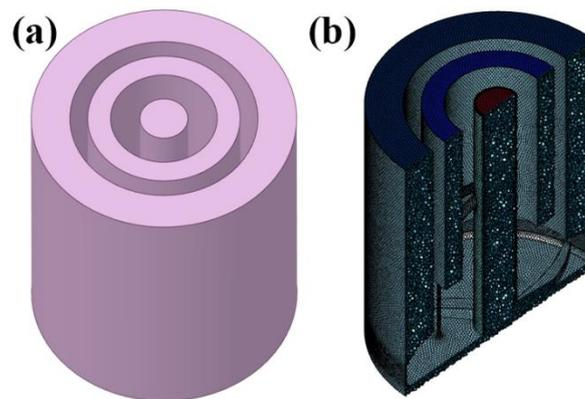
**Figure 3. Fluid Domain and Mesh Cell Section View**
