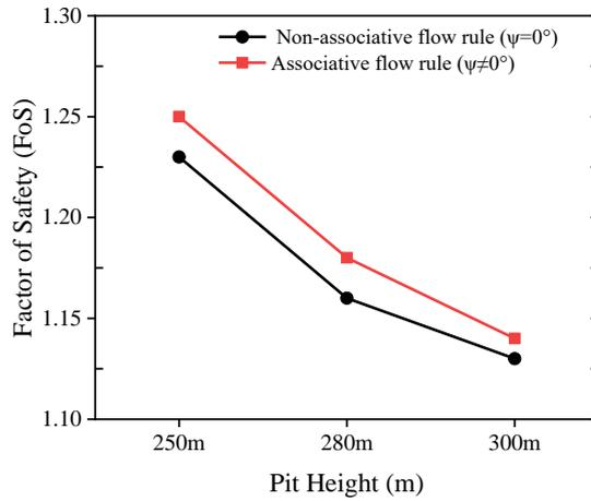
**Figure 4. Pit Stability Condition at Different Excavation Depth**
