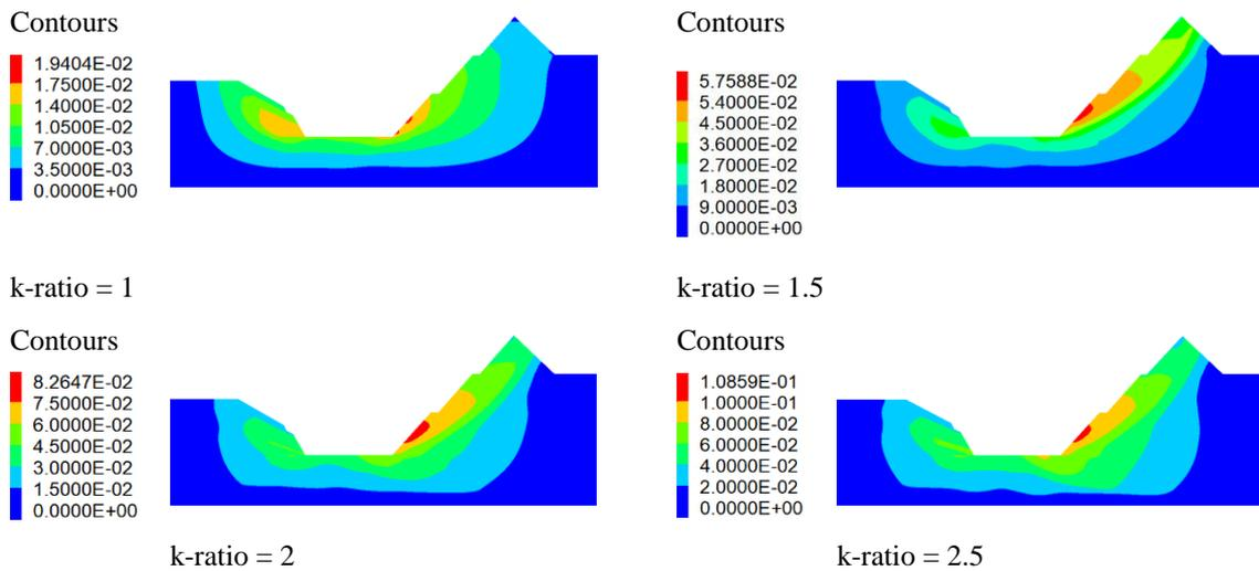
(b) Pit wall displacements at 280 m pit height
