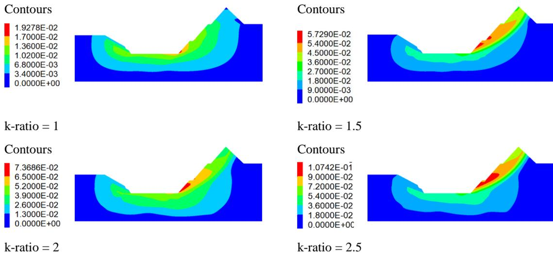
(a) Pit wall displacements at 250 m pit height
