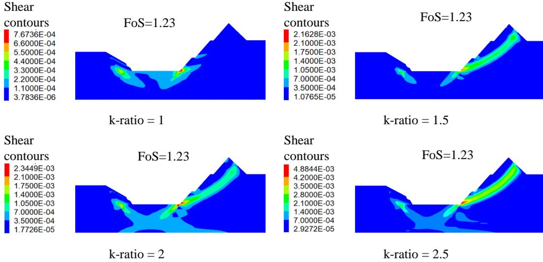
(a) Shearing pattern of pit walls at 250 m pit height
