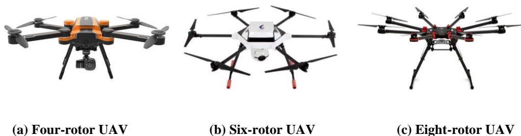
Figure 2. Common Multi-rotor UAV Types
