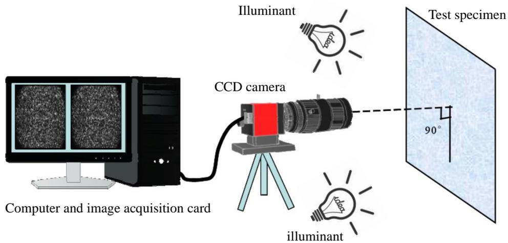
**Figure 1. Schematic Diagram of the VIC-3D Measurement System**
