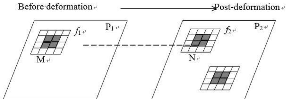
**Figure 2. Diagram of Subset Changes before and after Deformation**
