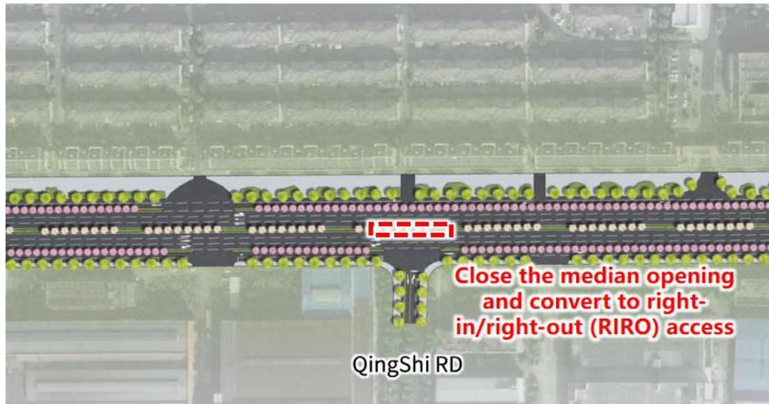
Figure 4.3-3 Schematic Diagram of Reducing the Opening of the Median Strip
